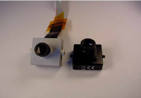
New camerahead for AXIS 209. Here we have to copy a analog camerahousing to replace it 1:1 with the 209.
