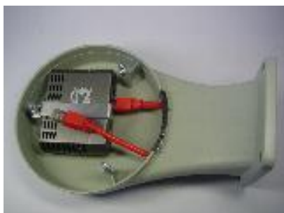
Wallmount 6102 with build in high PoE splitter
