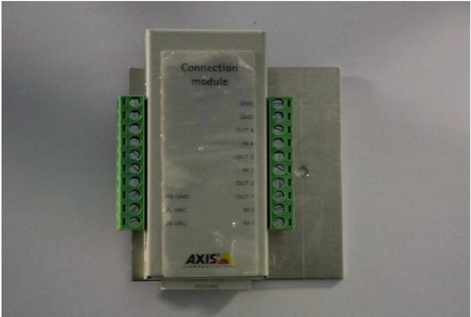
With the third screw you mount this unit now into the connector box on the shown position
