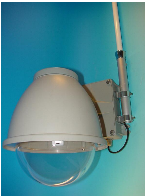
Build in W-Lan transmitter
