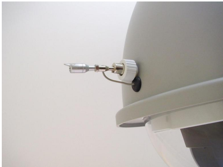
Build in outdoor microfon
